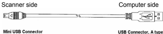
Now that the cable is connected to the scanner, connect the other side to your computer. Refer to the manual of your PC on how to do this. An A-type USB connector also fits in one position only, so when it does not easily slide into the PC, try to hold the connector upside down.
